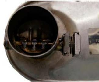
Figure 23. Prototype Exhaust Control Valve [13] with passive spring operation
