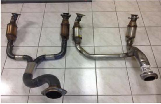
Figure 21. Equal Length versus Standard Y-pipe
