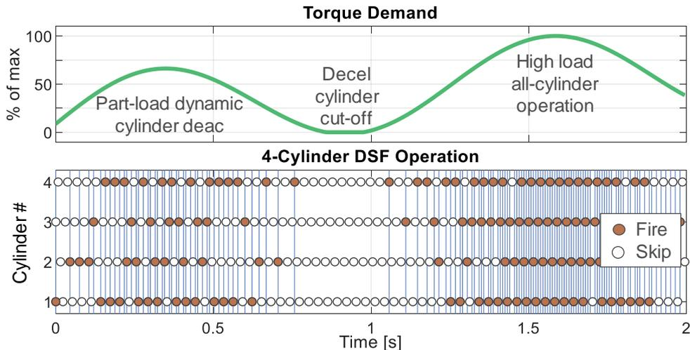
Fig. 1: DSF in a Transient Maneuver
