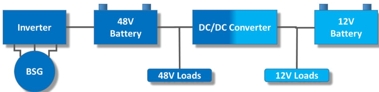
Fig. 8: Schematic Diagram of the 48V Mild Hybrid System Mechanization
