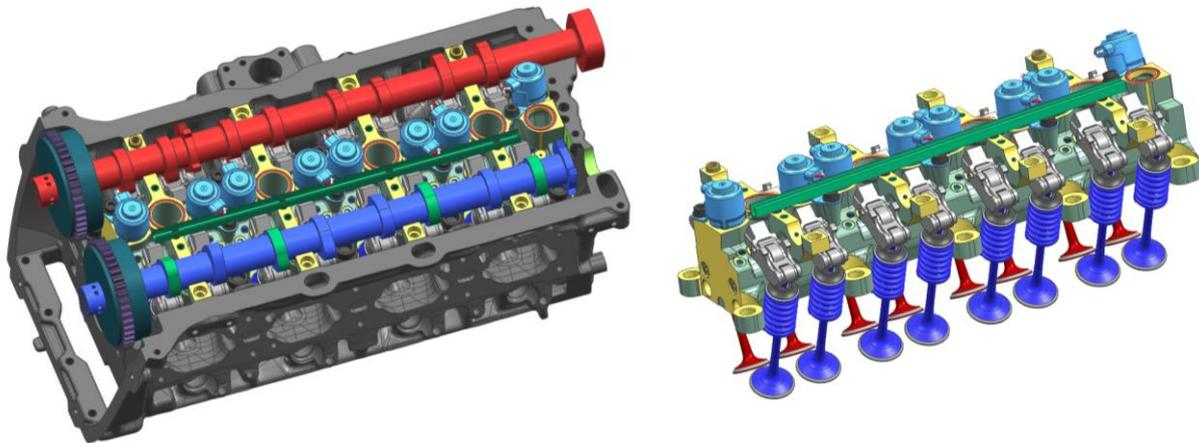
Fig. 20: Solid model of mDSF cylinder head using DSF cylinder deactivation hardware with 4 additional OCVs for independent intake valve control
