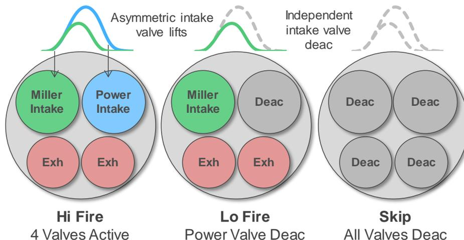
Fig. 19: Cost effective 3-state mechanization approach for mDSF using asymmetric intake ports and independent intake valve deactivation
