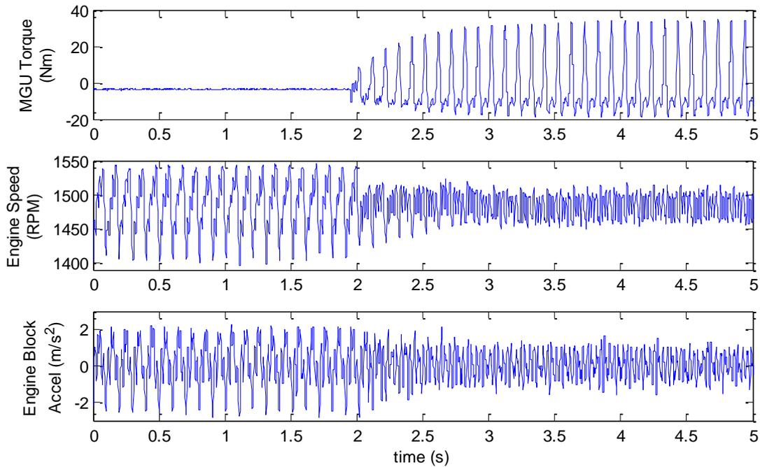
Fig. 14: eDSF Crank Torsional Variation Reduction Example, Time Traces
