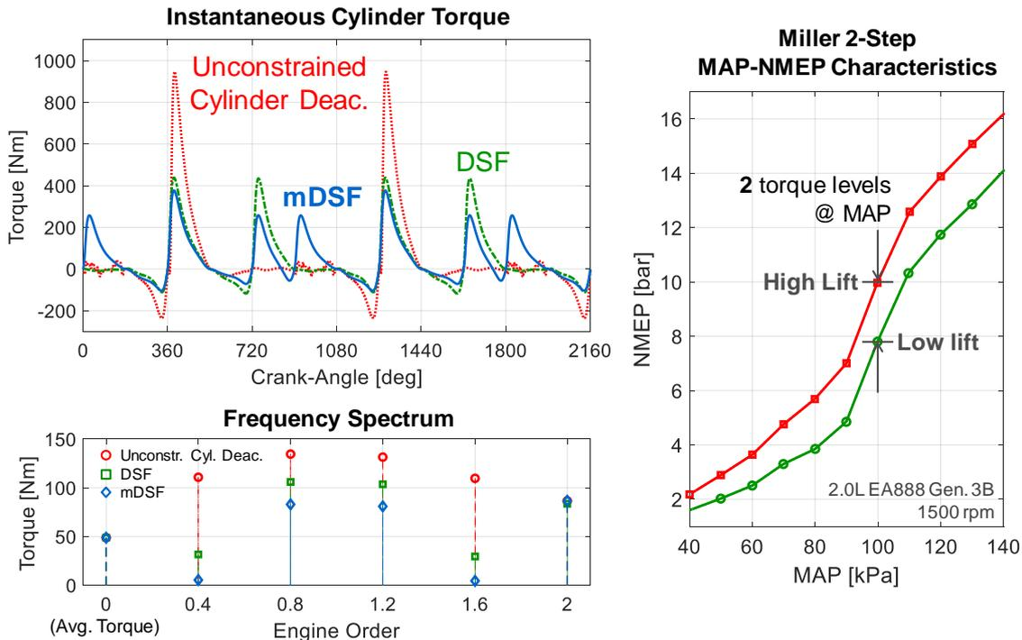
Fig. 17: NVH improvement opportunity presented by a 2-step Miller engine and exploited by mDSF to expand "flyzone" and maximize fuel efficiency benefit
