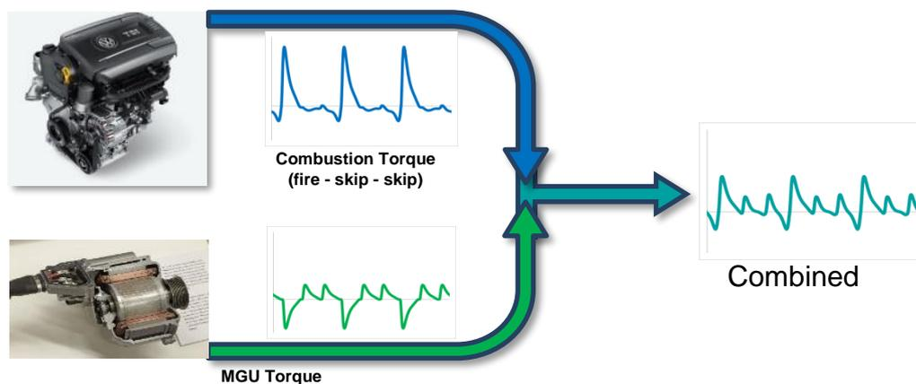
Fig. 6: Torque Smoothing Principle
