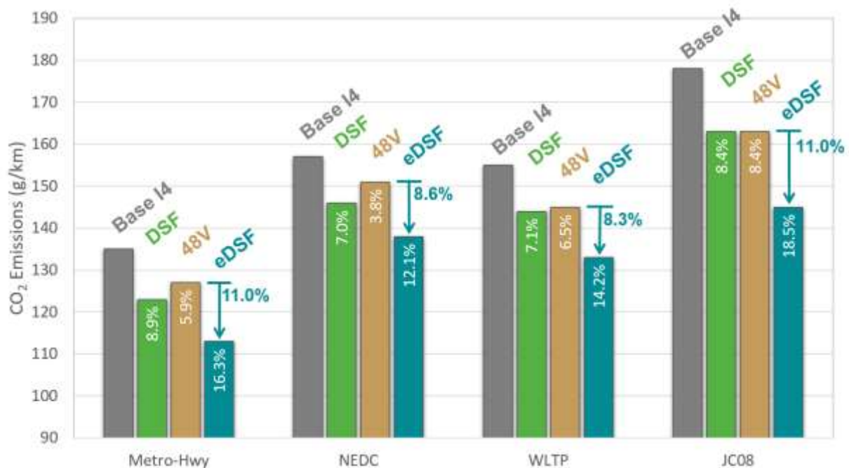
Fig. 6: CO 2 Emissions Reduction by Drive Cycle for DSF, All-cylinder with Mild Hybrid and eDSF vs. Base All-Cylinder Operation without Electrification
