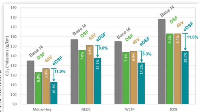
FIGURE 7 CO 2 Emissions Reduction by Drive Cycle for DSF, All-cylinder with Mild Hybrid and eDSF vs. Base All-Cylinder Operation without Electrification
