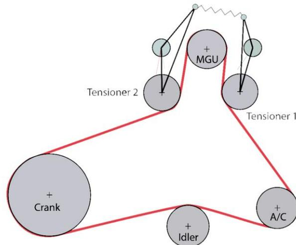
Fig. 11: Bidirectional FEAD Tensioner Arrangement
