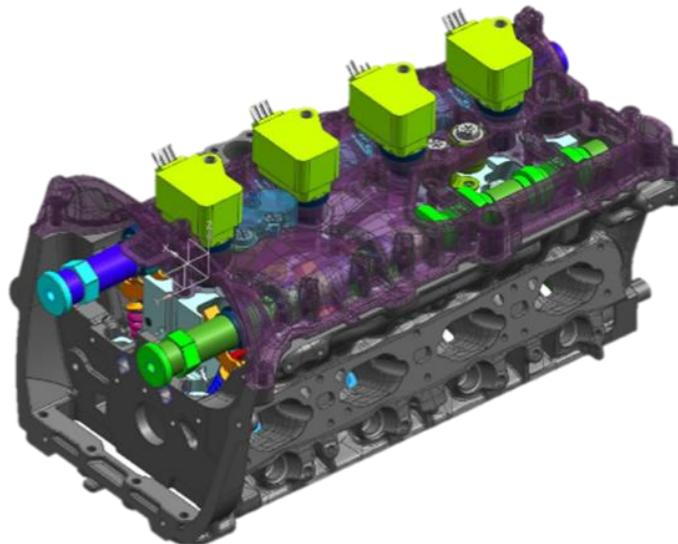
Fig. 2: Development DSF cylinder head with project specific hardware installed (modified casting, Deactivation Roller Finger Followers, Deactivation Control Valves, intake and exhaust camshafts and machined cam cover)
