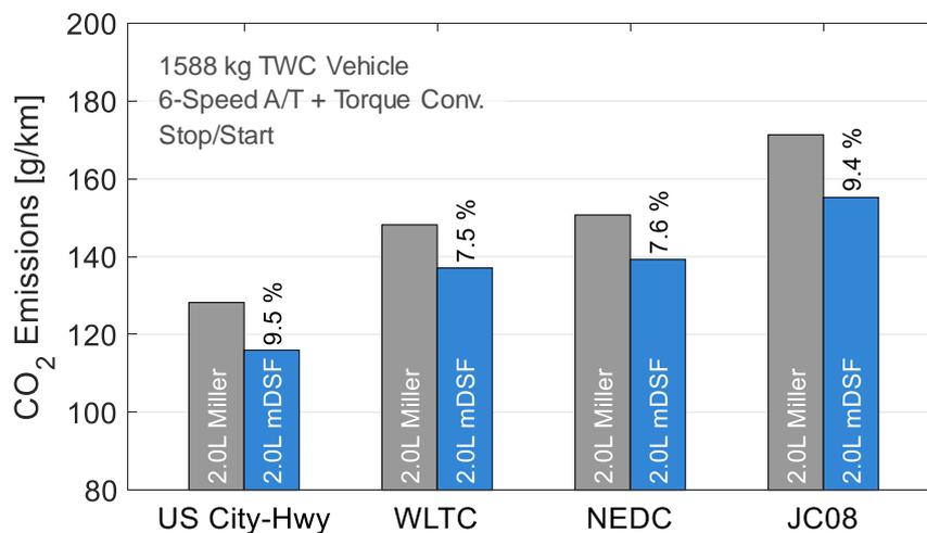
Fig. 23: mDSF vehicle CO<sub>2</sub> emissions in four certification drive cycles compared with baseline Miller 2-Step engine
