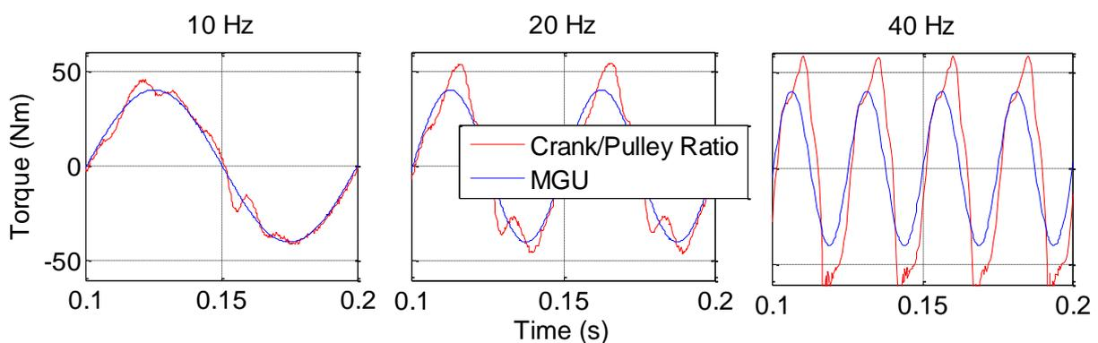
Fig. 12: Crankshaft Torque Responses to Sinusoidal MGU Torque Inputs at Various Frequencies
