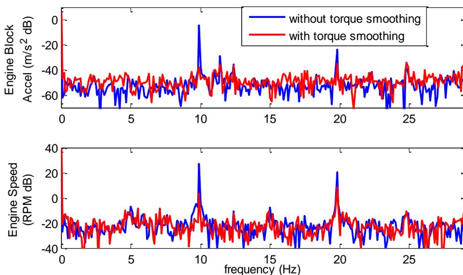
Fig. 15: eDSF Crank Torsional Variation Reduction Example, Spectra
