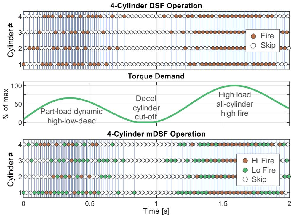
Fig. 18: Representative DSF and mDSF firing histories on a 4-cylinder engine for a changing torque request capturing low load, deceleration and high load operation
