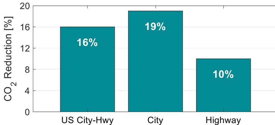
Fig. 9: Test results showing percentage CO<sub>2</sub> reduction results of 48V mild hybrid with eDSF system compared to the baseline vehicle
