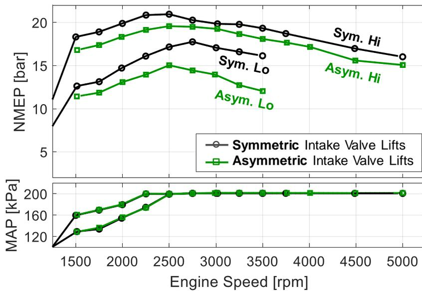
Fig. 21: Comparison of net torque output (NMEP) from symmetric and asymmetric intake valve lifts at constant manifold pressure (MAP)
