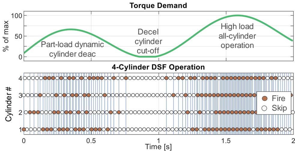
Fig. 1: DSF in a Transient Maneuver
