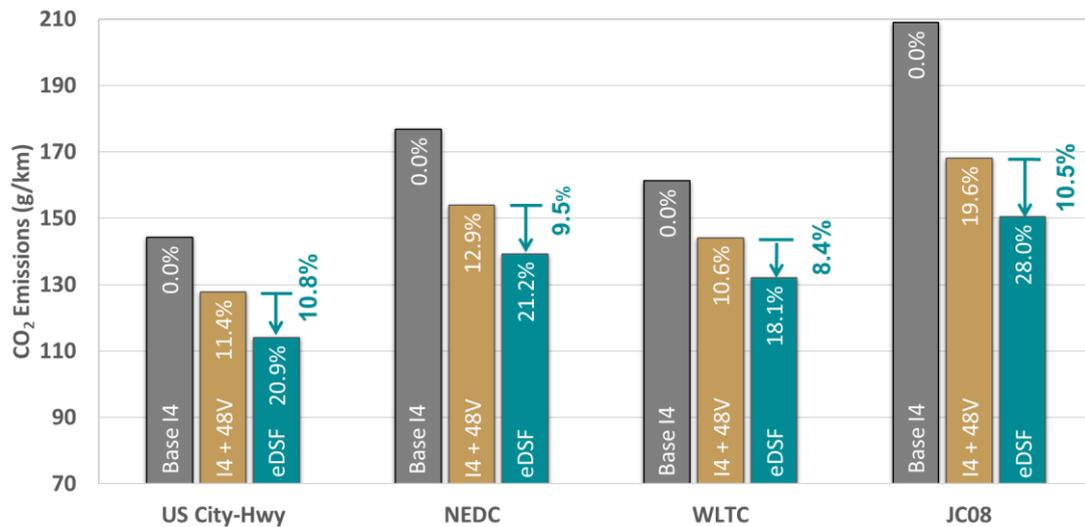
Fig. 16: CO<sub>2</sub> Emissions Reduction by Drive Cycle for DSF, All-cylinder with Mild Hybrid and eDSF vs. Base All-Cylinder Operation without Electrification
