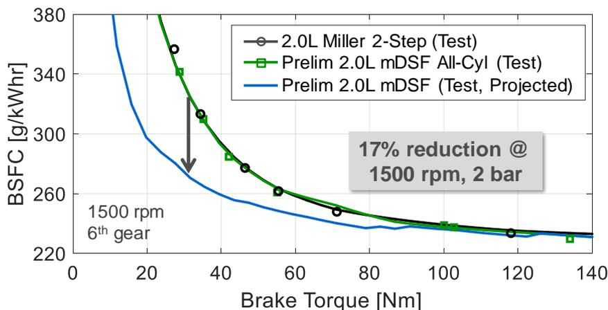
Fig. 22: mDSF engine fuel consumption compared with baseline Miller 2-step and mDSF all-cylinder (asymmetric valve lifts) at 1500 rpm, 6th gear
