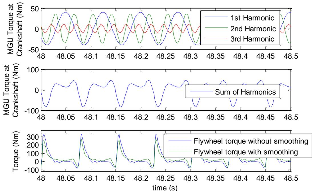
Fig. 13: Torque smoothing target waveform harmonics (top), sum of harmonics (middle), and flywheel torque before and after application of torque smoothing (bottom)
