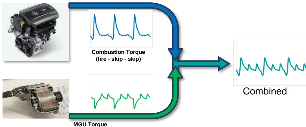
Fig. 6: Torque Smoothing Principle
