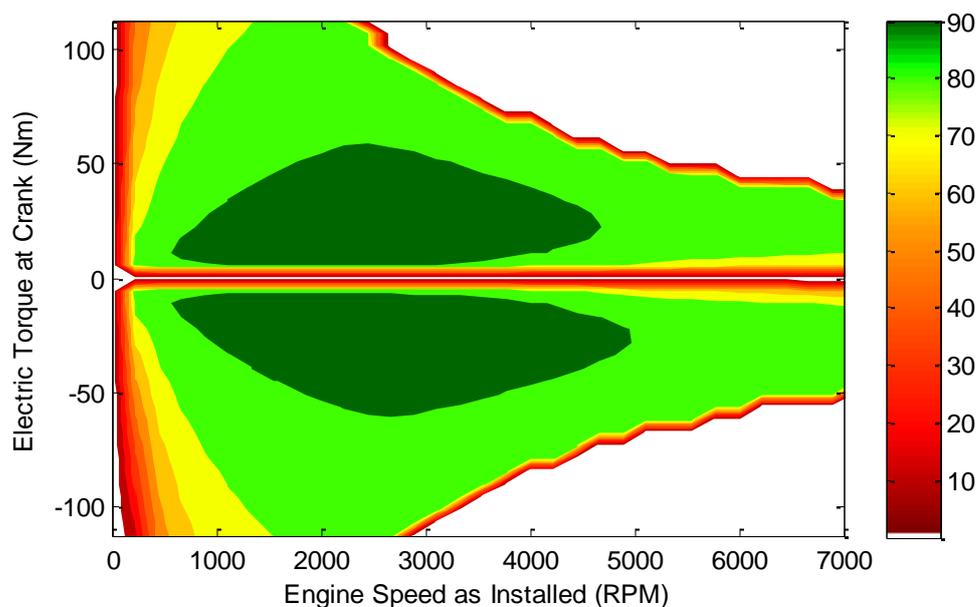
Fig. 10: PMSM Inverter Integrated Efficiency Map Example
