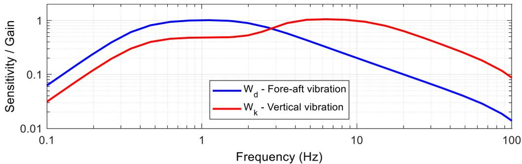
Fig. 5: ISO 2631 Standard Weighting Functions for Human Sensitivity to Vibration
