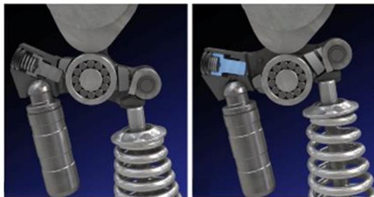
Fig. 4: Deactivation Roller Finger Follower at peak cam lift, in Activated (left) and Deactivated (right) states
