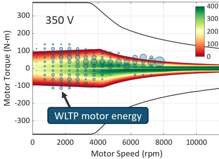
Fig.5 Simulation results of DMD loss reduction in Watts at 350V battery voltage of an 142kW EESM and energy consumption of the motor and inverter system in the WLTP drive cycle.
