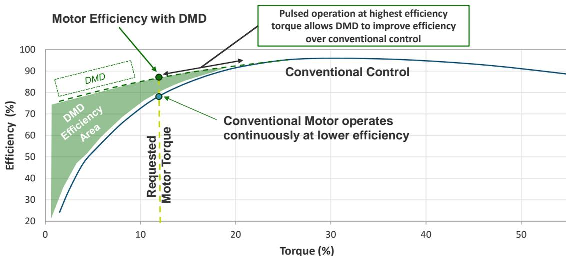
Fig.1 A typical motor system efficiency characteristics at a constant speed.
