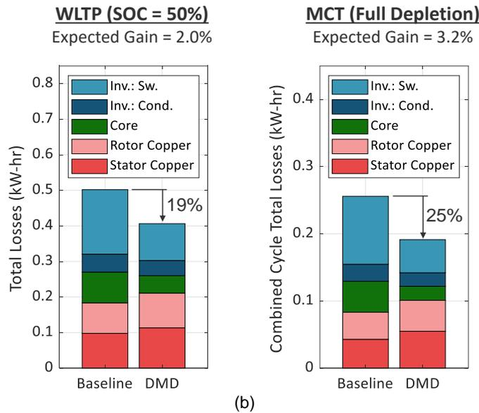
Fig.6 Loss breakdown and reduction amount of DMD in the WLTP and MCT drive cycles.
