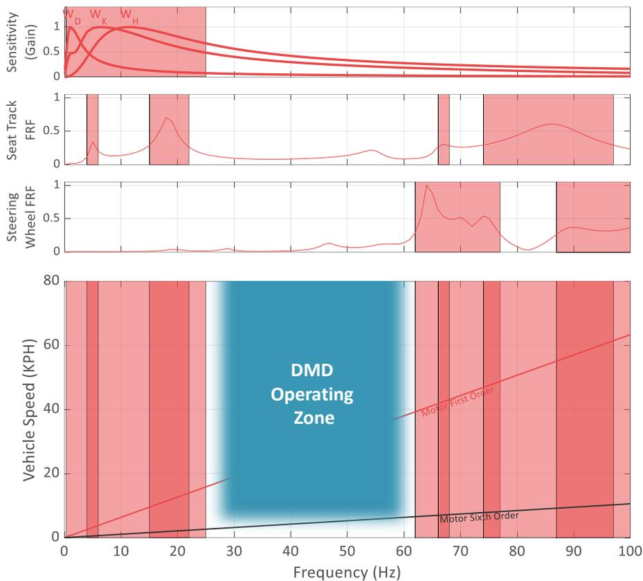
Fig.4 DMD algorithms operates while avoiding resonances and perceptible vibration. (a) top: human sensitivity gain; (b) middle: frequency response functions at seat track and steering wheel for a 2020 Chevrolet Bolt; (c) bottom: DMD operating zone.
