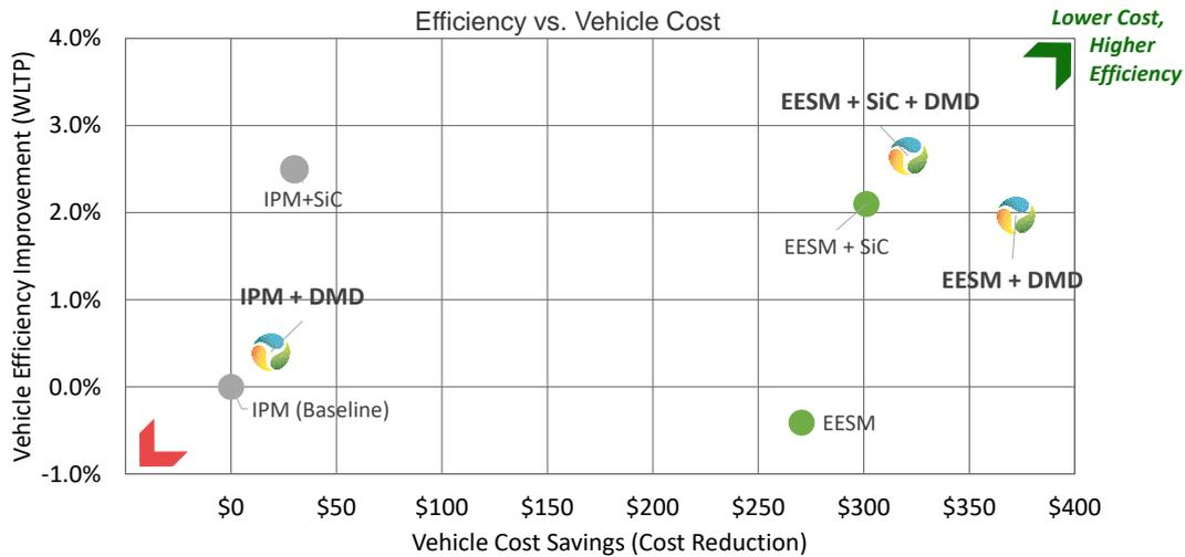
Fig.7 The impact of DMD on an IPM and an EESM for traction drives.
