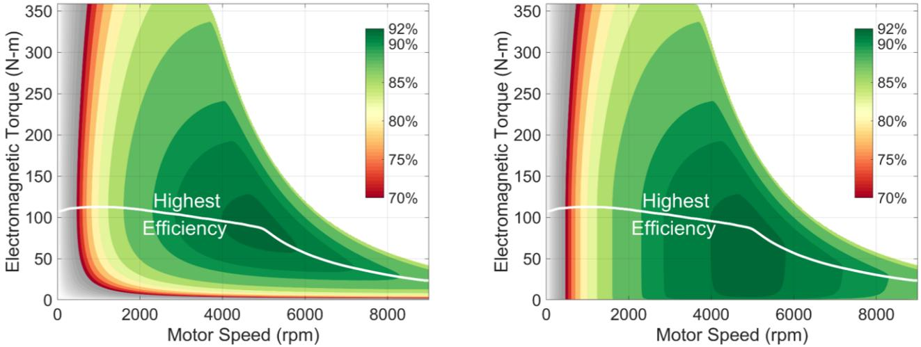
Fig.2 Improved electrical efficiency at low loads from conventional control (left) to DMD (right).
