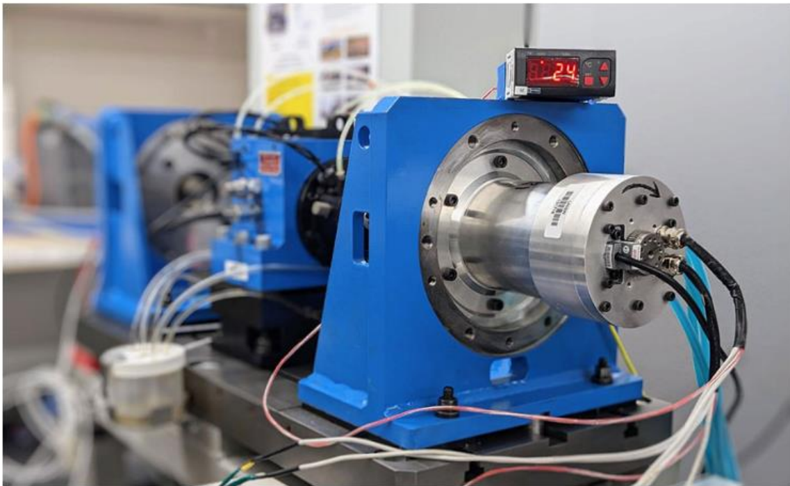
This motor achieves high efficiency and high power density with reduced rare-earth magnets. Photo courtesy the University of New South Wales
