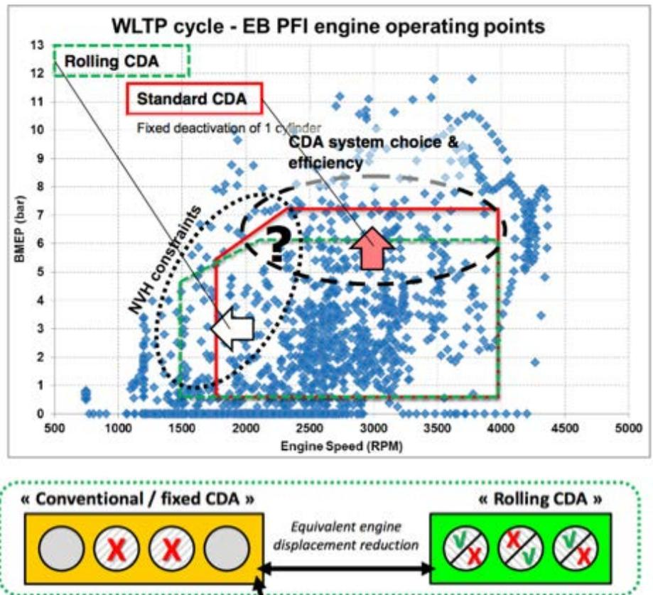
**Figure 2.** Eaton and PSA, Dynamic Cylinder De-Activation: System approach and performance potential. (Source: Ceur, Majo, Veiga-Pagliari, D.R. “Dynamic Cylinder De-Activation (D-CDA).” PSA & Eaton. Presented at 24th Aachen Colloquim Automobile and Engine Technology. October 7, 2015. Slides 4-5.)
