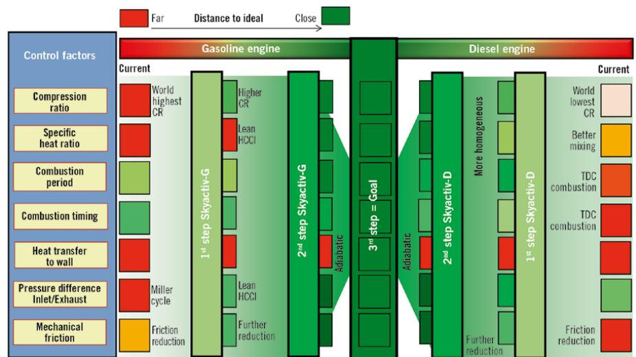
**Figure 3.** Mazda map for incremental improvements in gasoline (and diesel) engines. (Source: Hirose, Ichiro, Hitomi, Mitsuo. “Mazda’s Way to More Efficient Internal Combustion Engines.”)
