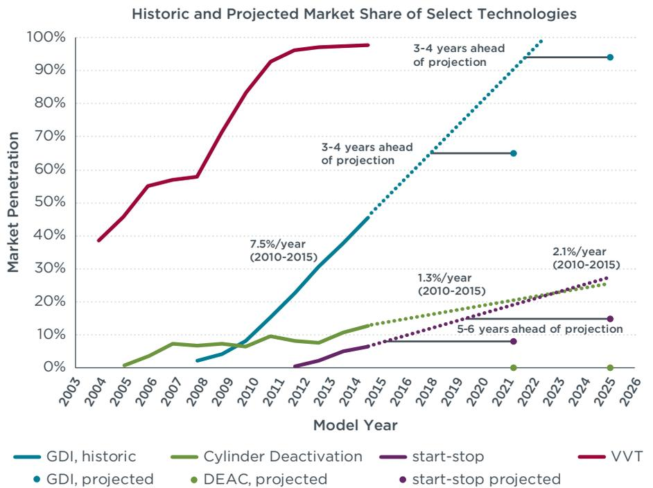
**Figure 4.** Market penetration of select technologies, and extrapolation to rulemaking (RM) projected penetration. Based on U.S. EPA fuel economy trends report for 2015. Note that the 2015 values are estimates.
