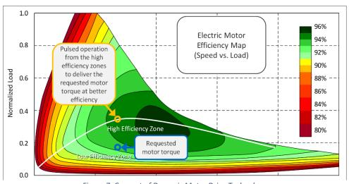
Figure 7: Concept of Dynamic Motor Drive Technology
