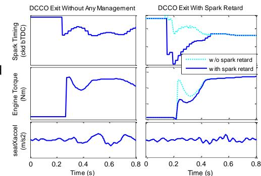
Brief DFCO period at the end of DCCO reduces manifold pressure and combustion torque on refiring
